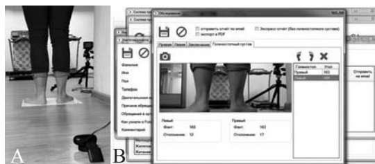
Figure 9.—Photography of the ankle joint: A) position of the web camera and the athlete (length: 0.8 m); B) estimation of the foot-ankle angle.
